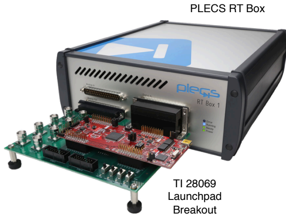
Figure 6: Hardware setup of the HIL verification
