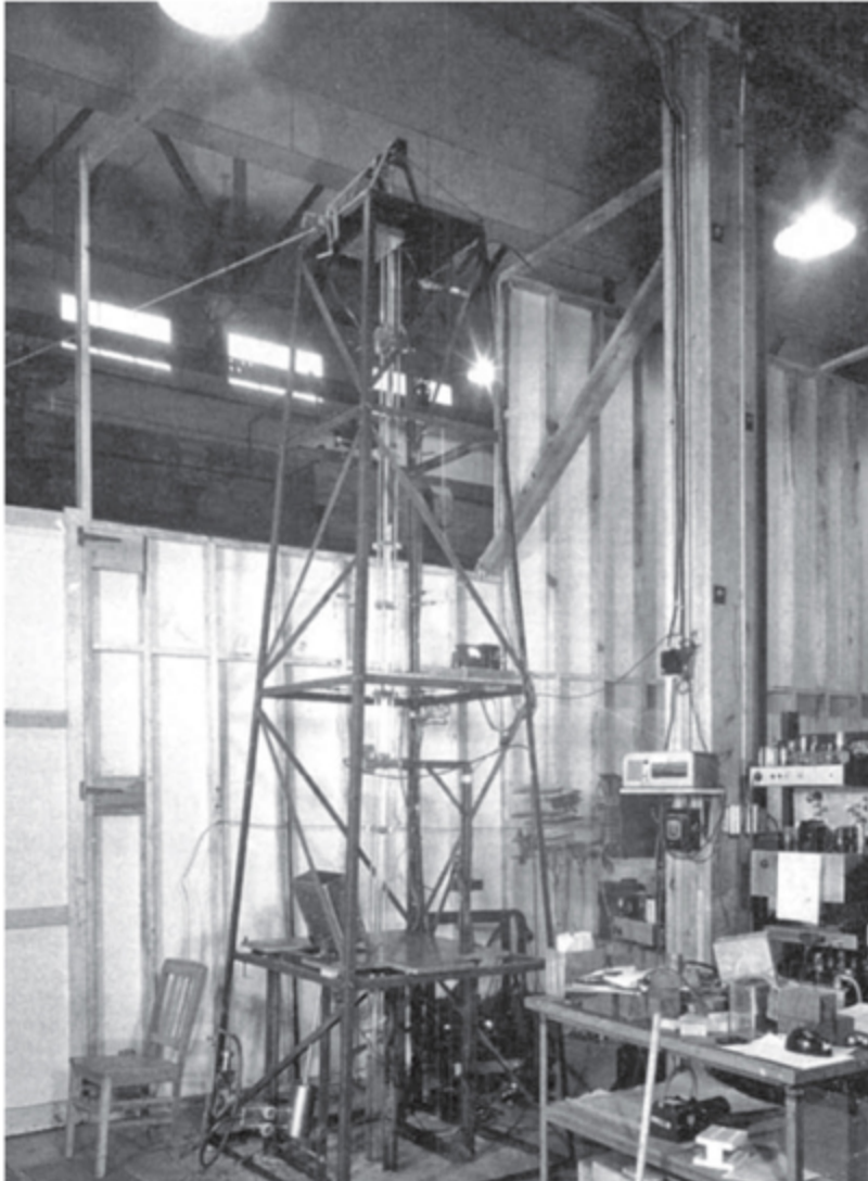
Guillotine mechanism for studying supercritical assemblies, the Dragon experiment. Gravity pulled pieces of metal hydride down a wire through rings of the same material. Theoretical physicist Richard Feynman said it was like tickling the tail of a sleeping dragon. Courtesy of Los Alamos National Laboratory.
