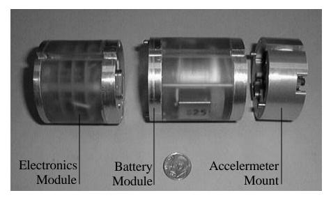
Figure 1: Photograph of MinPen Acceleration Recorder
