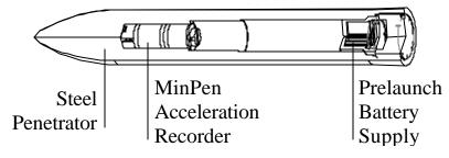
Figure 4: MinPen secured inside Penetrator
