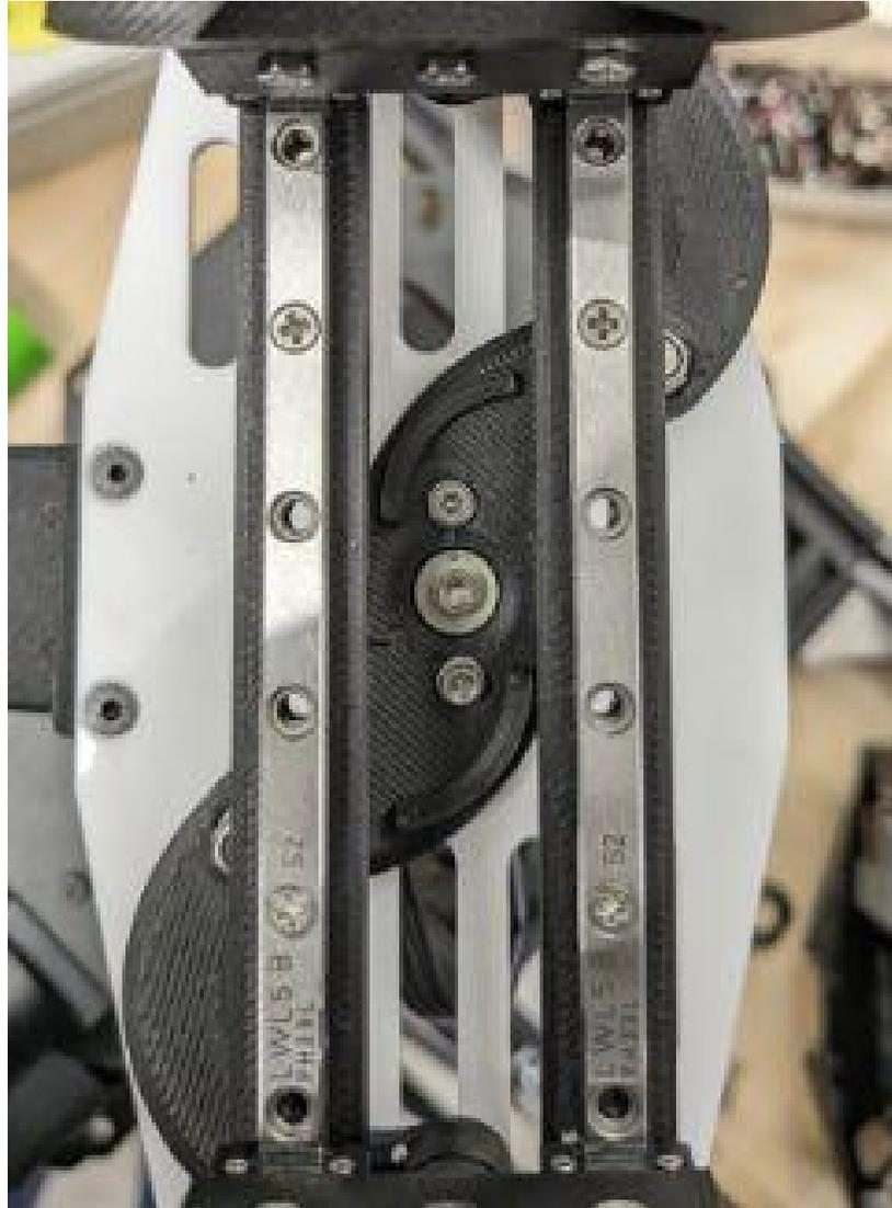
Step 15: Move the finger open and close to ensure smooth movement. The gripper assembly is now complete.
