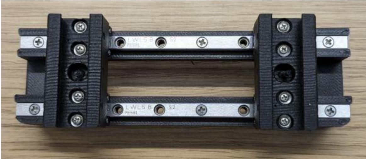
Step 8: Use M3x 20mm countersunk screws to attach the rotor-link to the finger adaptor.
