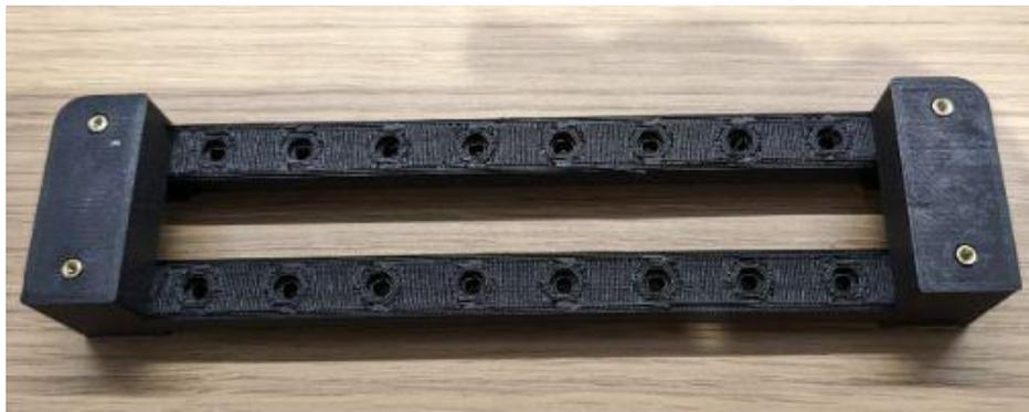
Step 2: After laser cutting 3mm acrylic, countersink the holes as shown in the picture.
