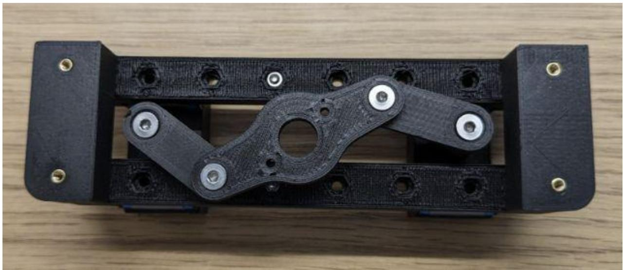
Step 9: Attach the backplate to the bridge using M2 x 10mm screws, making sure the countersunk holes are facing forward. To ensure the backplate is correctly oriented, check that the center of the large holes are aligned with the center of the two rails.
