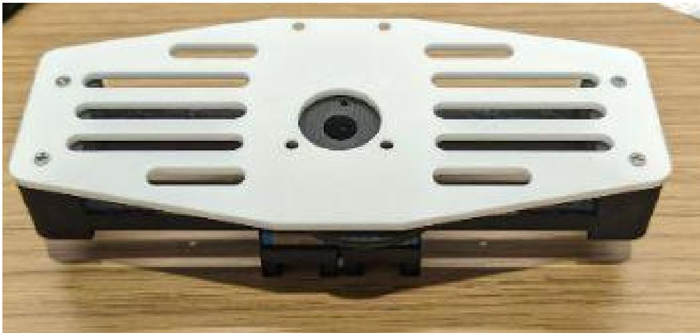
Step 10: Move the finger adaptor open or closed to ensure that the rotor rotates correctly (close = clockwise, open = counterclockwise).
