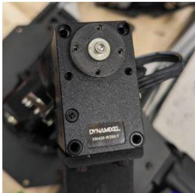
Step 14: Use an M2x6mm screw and washer to secure the rotor to the motor horn. Use M2.5x16 countersunk screws to secure the gripper to the motor. Make sure the orientation is correct according to your configuration.
