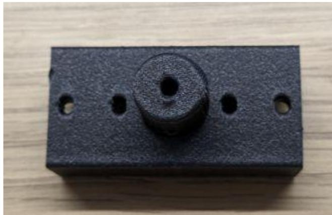
Step 5: Attach the rotor and rotor arm together with an M3x10mm countersunk screw and lock nut, as shown in the figure.
