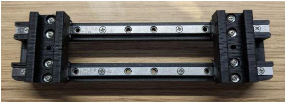
Step 8: Use M3x 20mm countersunk screws to attach the rotor-link to the finger adaptor.
