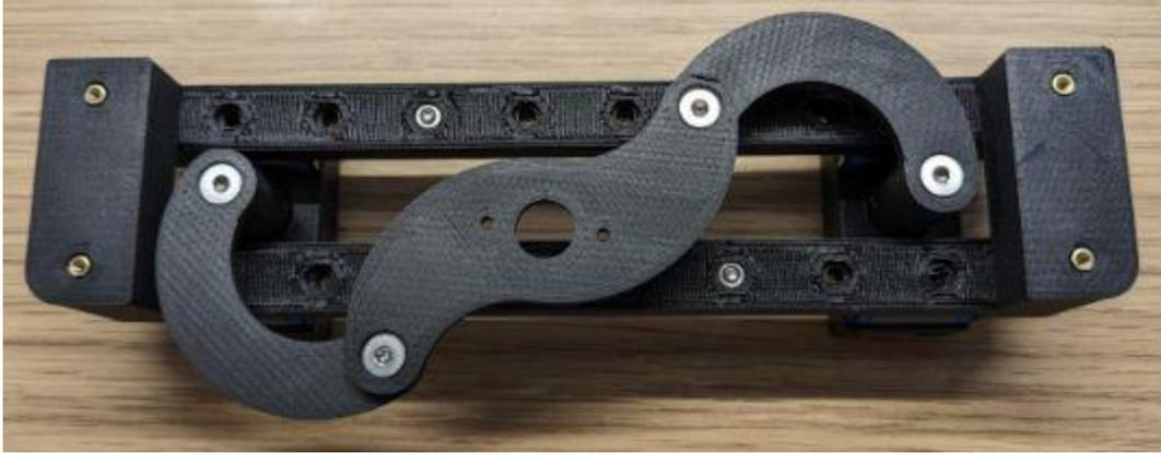
Step 9: Attach the backplate to the bridge using M2 x 10mm screws, making sure the countersunk holes are facing forward. To ensure the backplate is correctly oriented, check that the center of the large holes are aligned with the center of the two rails.
