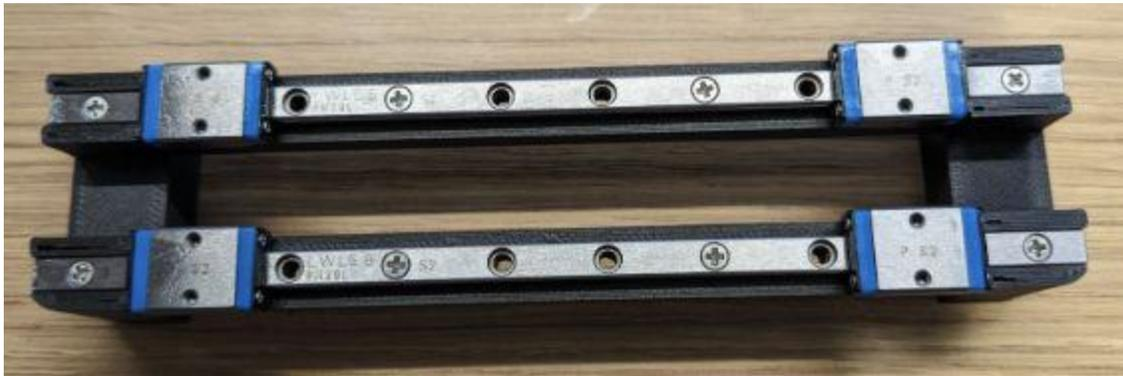
Step 7: Attach the finger adapter to the carriages using the 8 button head screws (6mm) that came with the rails and small OD flat washers.
