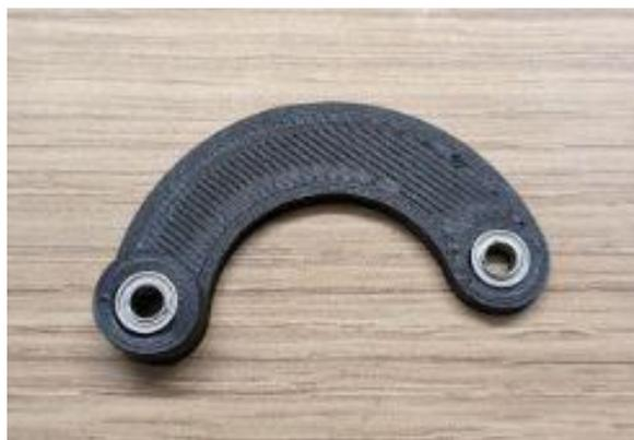
Step 4: Use a tap to create M3 threads in the middle holes, to a depth of about 5mm.
