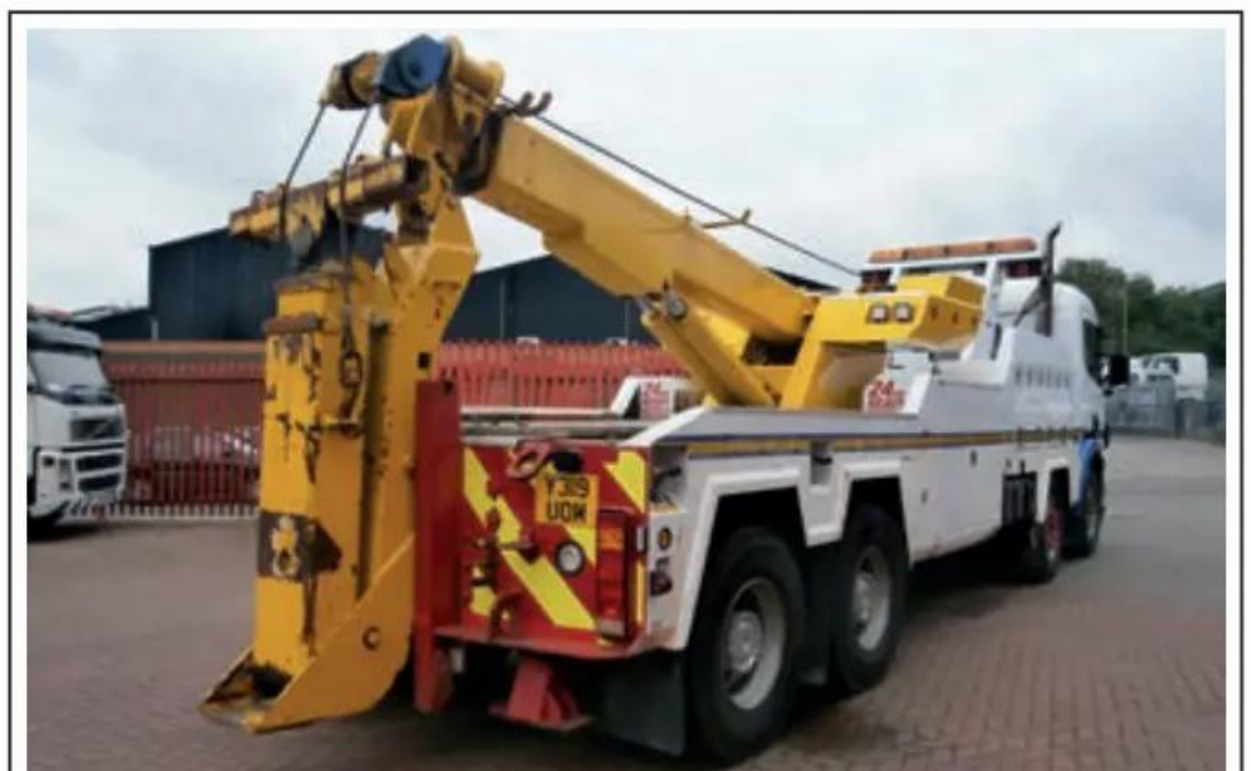
Scania P124C 8x4 , 420 engine, manual gearbox, dual winches, 3 stage crane boom, remote control, Equipped ready to go NRC underlift, boom, New Test – SV6120
