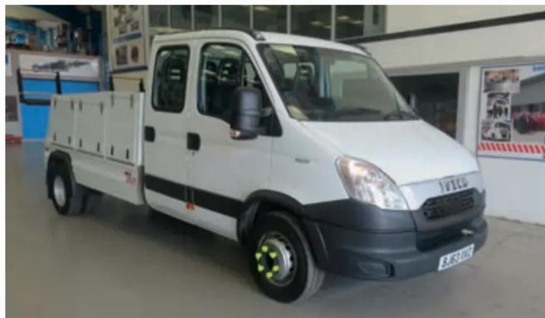
Iveco 70C18D With Dyson Enforcer wheel lift full hydraulic with H8 hydraulic winch, full plastic body lockers, choice of two, 2013, 63 Reg & 2014, 64 Reg – SV6274/5
