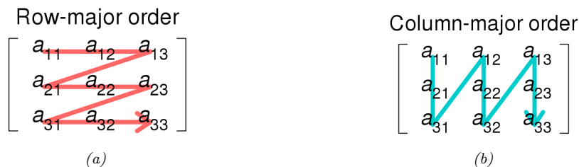
Figure 7.2: Illustration of (a) row-major vs (b) column-major order. From https://commons.wikimedia.org/wiki/File:Row_and_column_major_order.svg . Used with kind permission of Wikipedia author Cmglee.
