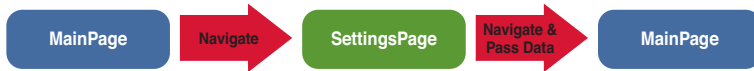
FIGURE 7.8 Simulating the return of data by navigating forward to the page on the back stack.
