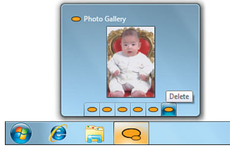
FIGURE 15.2 Applying the same EllipseGeometry to a Window’s icon, taskbar item overlay, and all its thumb buttons.
