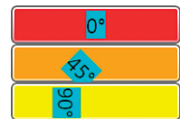
FIGURE 4.10 Inner TextBlocks rotated around their top-left corner, with an explicit background.
