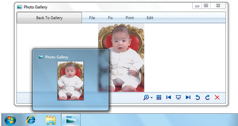
FIGURE 8.15 Clipping the taskbar thumbnail to a photo rather than the entire window.
