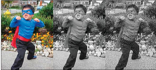
FIGURE 11.2 Displaying an Image with three different pixel formats.
