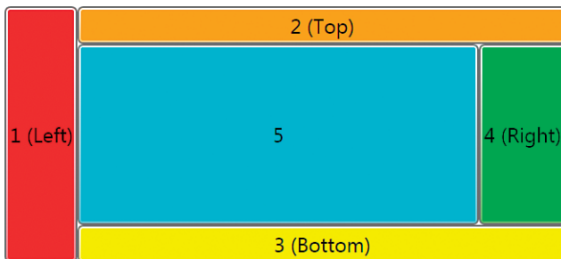
FIGURE 5.8 Buttons arranged in a DockPane1 in a different order than Figure 5.6.
