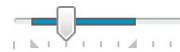
FIGURE 11.23 Slider supports a selection range that can be a subset of the main range.
