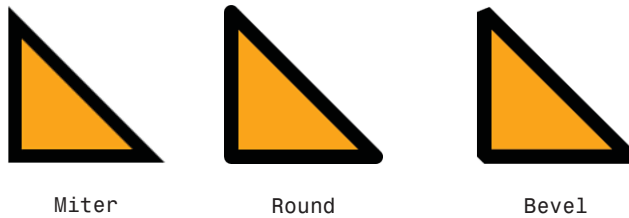
FIGURE 15.11 Each type of LineJoin applied to the familiar triangle.
