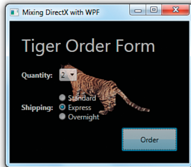
FIGURE 19.11 A WPF Window containing a DirectX-based spinning 3D tiger underneath basic WPF controls.
