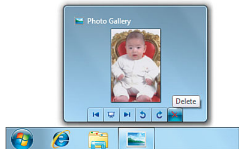
FIGURE 8.16 Thumb buttons can be placed inside the thumbnail preview popup.
