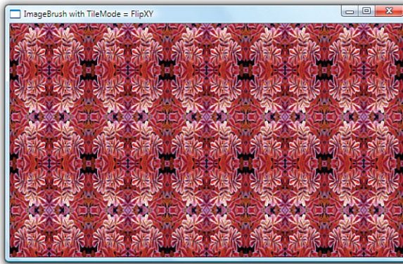
FIGURE 15.36 The ImageBrush background, using TileMode=FlipXY to create an interesting pattern.
