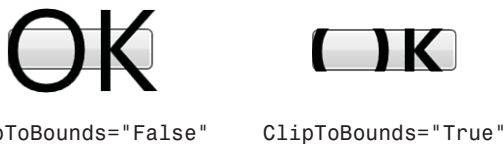
FIGURE 5.19 ClipToBounds can be used on a control such as Button to affect the rendering of its inner content.
