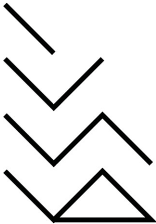
FIGURE 15.18 Four Polylines , ranging from 2 to 5 points.
