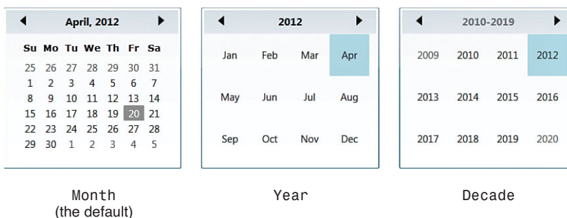
FIGURE 11.24 The WPF Calendar , displayed with each of its DisplayMode values, as it appears on April 20, 2012.
