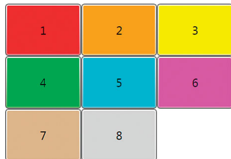
FIGURE 5.17 Eight Buttons added to a UniformGrid .
